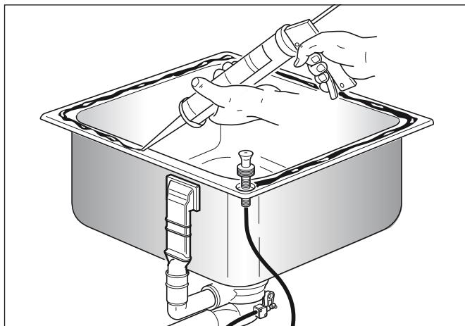
2. In order to avoid water infiltration, apply some sealant on the bowl's rim. Push the bowl against the underlying part of the countertop.
