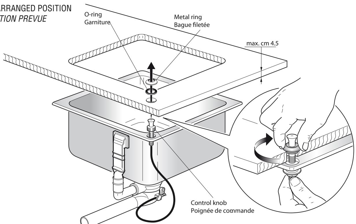
If necessary, the control knob can be positioned further away from the bowl's rim.
