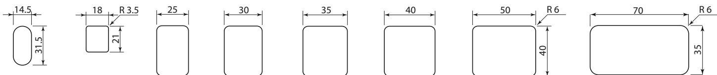
DIMENSIONS AND POSITION OF CONTROL KNOB AND TAP INSTALLATION CUTOUTS
